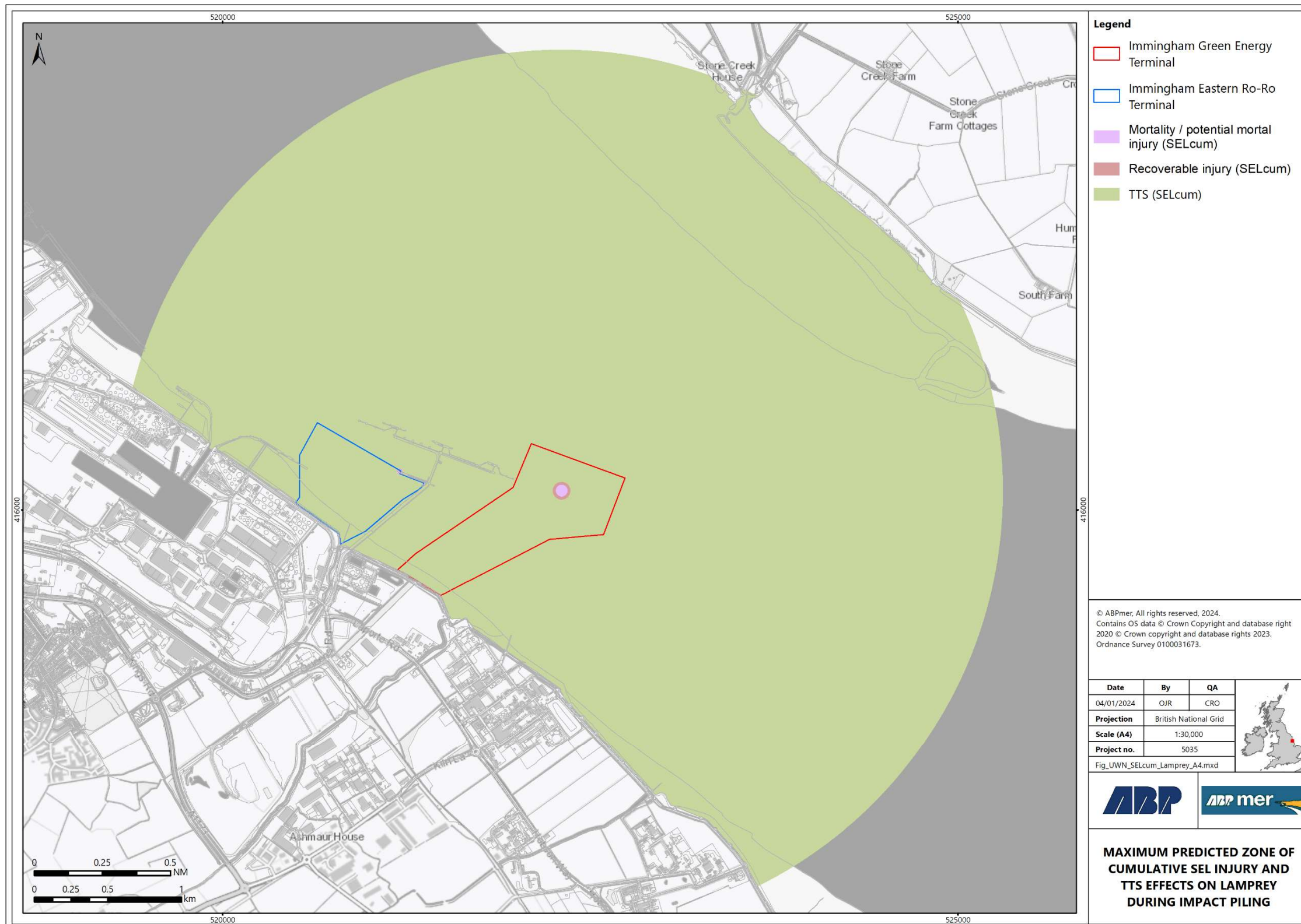
Figure 2. Maximum predicted zone of cumulative SEL injury and TTS effects on lamprey during impact piling
